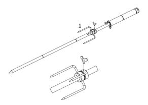
4. Screw the first tripod (1) to the motor's connecting pin. Connect the other tripod (2) to the skewer's edge.
